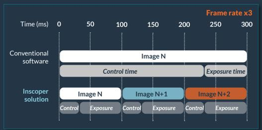
The INSCOPER approach involves embedding Device Control in a specialized electronic unit. This unit has been designed to communicate with devices in the same way as hardware to control them as quickly and reliably as possible. This solution eliminates all latency caused by the operating system (Windows) and the multiple software drivers it requires to communicate with devices.
